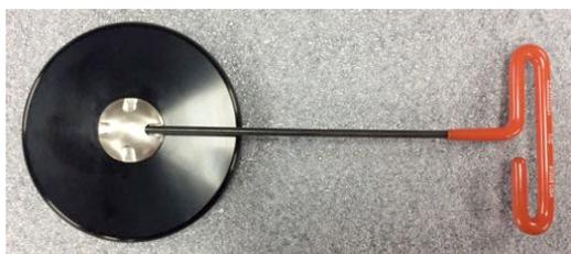
$\frac{1}{8}$ " T-wrench inserted into the adjustable screw
